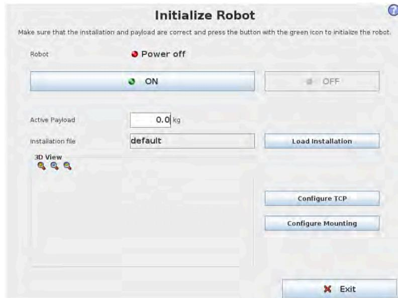
**f** Tap **START** to release the brakes. The robot will make some clicking sounds and small movements.
