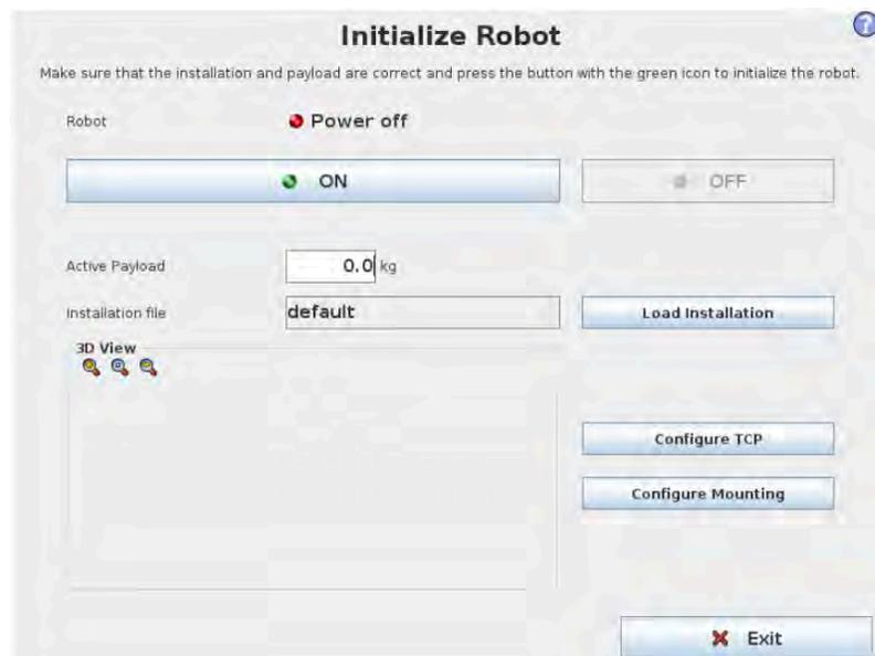
**d** Set your Tool Center Point (TCP), payload, and center of gravity. The settings save when you tap **Exit**.
