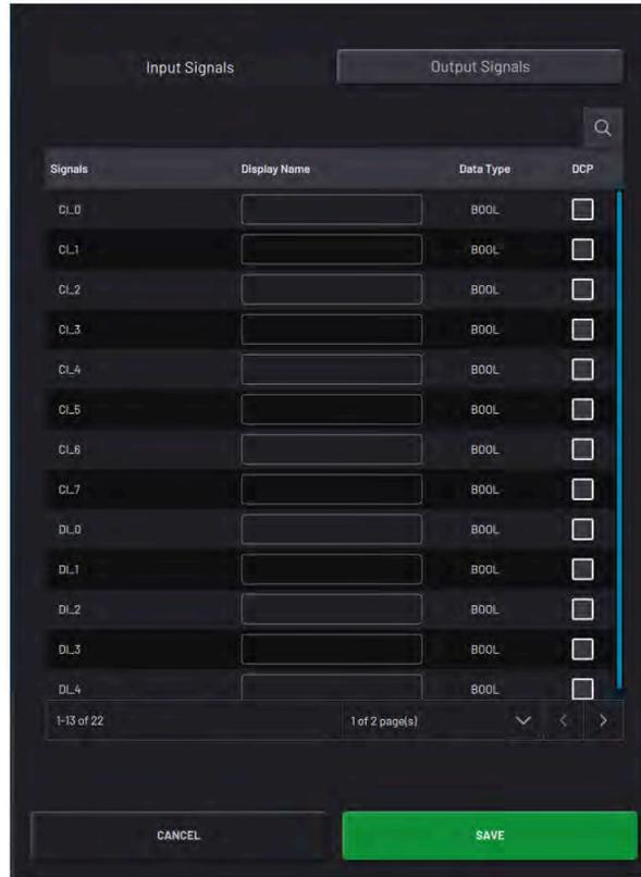
**a** Enter a **Display Name** (i.e. "Open Machine Door", "Open Pneumatic Vise", or "Start Machining Cycle") to show what each signal does in other apps.
